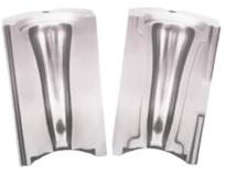
Substitution of HVOF coating for PVD Shorter cooling cycle 30% cooling energy savings
